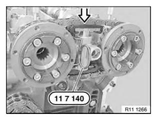
Compress secondary chain tensioner at top and remove special tool 11 7 140 .
