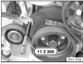
Crank engine at central bolt in direction of rotation until 1st cylinder is at TDC firing position. Secure vibration damper in position with special tool  $11\ 2\ 300$  .
