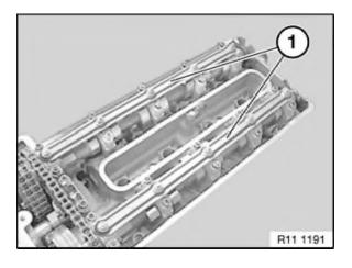
Remove oil lines (1) from cylinder head on cylinder banks 1 to 4 and 5 to 8.
