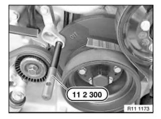
"No" screws are inserted in inlet sprocket wheel yet. Inlet sprocket wheel must not slip off centering sleeve.
