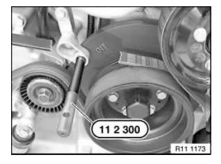
Rotate crankshaft in direction of rotation as far as ignition TDC position of cylinder 1. Secure vibration damper in position with special tool 11 2 300 .
