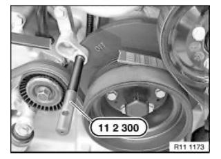
Then crank engine again in direction of rotation until 1st cylinder is at TDC firing position.
