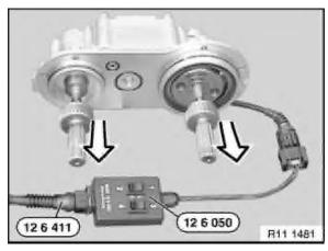
Connect special tool 12 6 050 in conjunction with special tool 12 6 411 to solenoid valves of VANOS adjustment unit. Connect special tool 12 6 411 to correct terminals on car battery.
