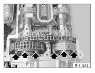
Slacken six accessible bolts two turns.
