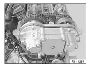
Cylinder bank 5 to 8: Attach VANOS adjustment unit.
