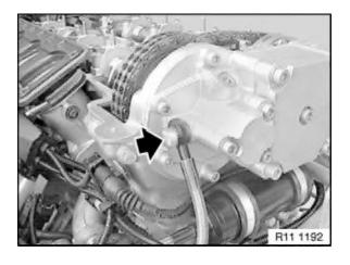
Cylinder bank 5 to 8: Remove oil line from VANOS adjustment unit.
