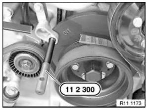
Rotate crankshaft in direction of rotation as far as ignition TDC position of cylinder 1. Secure vibration damper in position with special tool  $11\ 2\ 300$  .
