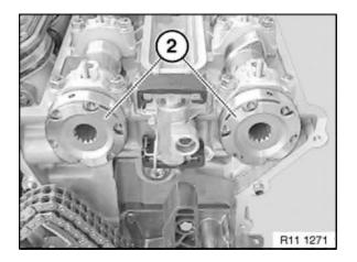
Withdraw toothed sleeves (2) from exhaust and inlet camshafts.
