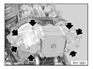
Cylinder bank 5 to 8: Release screws on VANOS adjustment unit.
